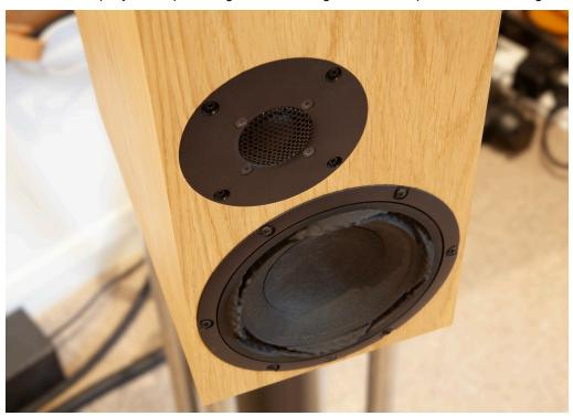
of quality control. The purpose of this change is to give the tweeter easier freedom of movement, the standard aluminium voice coil has a small magnetic braking effect which slows its response enough to make an audible difference in Joakim's opinion. He is not alone in thinking this way, it's an approach found in a number of high end tweeters used by larger brands.
